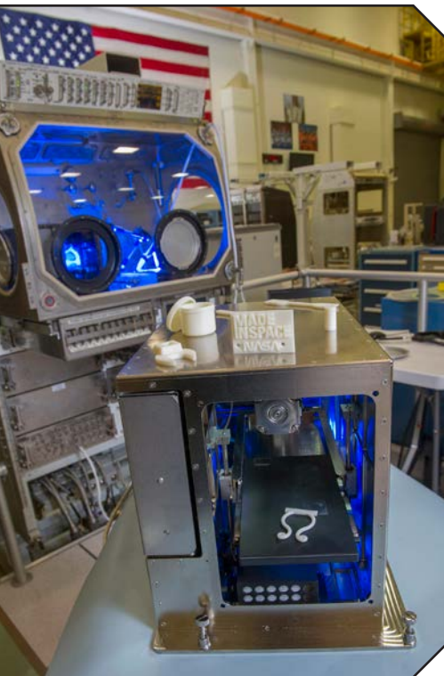
Made In Space's NASA-contracted, first 3D printer, was sent to the ISS on September 21st, 2014. The ivory objects on top are duplicates of what will soon be some of the first objects ever printed off-Earth. In the background is the Microgravity Science Glovebox that will contain the printer during the 3D Printing in Zero-Gravity Experimentation (Photo: NASA/Emmett Given).
