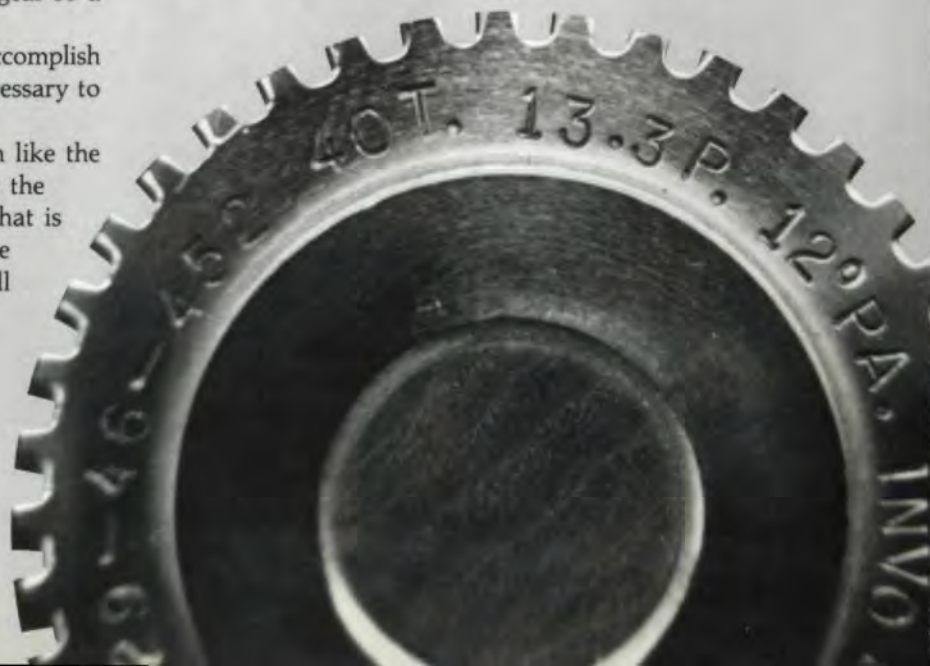
Fig. 3—This photograph shows an actual master gear which has proportions similar to those shown in Fig. 2. The method outlined chose a measuring ball size without difficulty.
