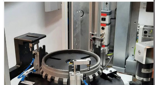
Mahr MWF GmbH Develops Measuring Machine for Double-Flank Gear Roll Testing
