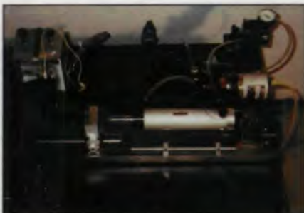
Fig. 8—Transmission testing device with computer controlled air cylinder and load cell.
