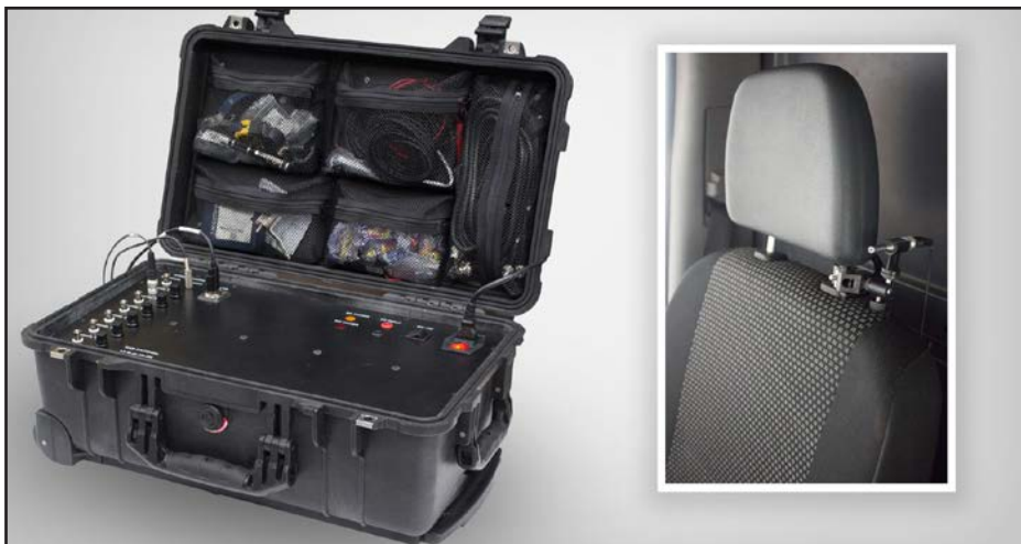
Figure 2 Authors’ in-house hardware solution for noise/vibration testing and transmission error testing, showing portable hardware used within project.
