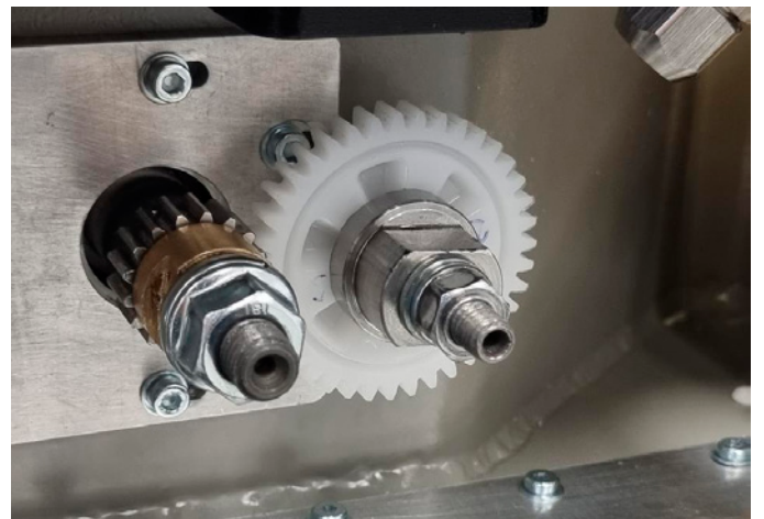
Figure 13—A combination of a steel pinion and a plastic gear is usually employed for the S-N curve generation. As the purpose of testing is to generate fatigue data on the selected plastic material, the failure needs to occur on the plastic gear. In a plastic/plastic configuration, the failure would be impossible to control, usually, both gears get damaged at the end of the test. Furthermore, the load-induced contact ratio increase would be even higher for a plastic/plastic gear configuration.
