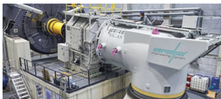
Figure 14—Test of the drive train under torque and bending load. Blue part in the background: E-motor to generate the torque load. Yellow part: torque coupling. Grey box with angled top: device to apply bending moments (Ref. 9).
