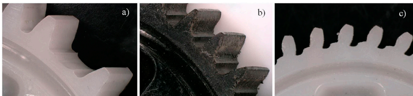
Figure 1—Possible failure modes for plastic gears: a) root fatigue, b) wear, c) viscoplastic deformation at thermal overload.
