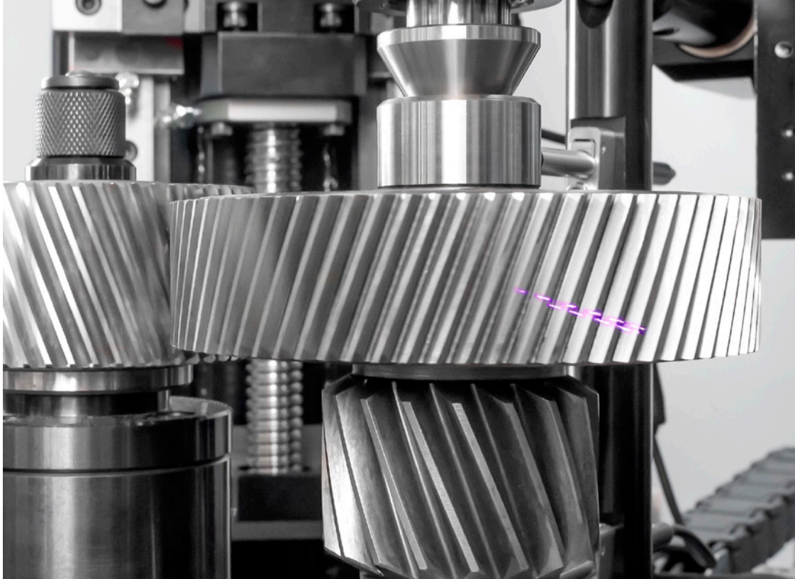
GRSL rolls multiple inspection methods into a single platform: optical inspection of profile, lead, and pitch; DOP and tooth thickness; double flank composite testing; and sophisticated in-process gear noise analysis.
