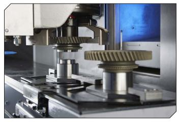
The pick-up automation system is the platform for the success of EMAG machines. Every machine in the VLC series features a parts storage area for raw and finished parts, as well as a working spindle that is automatically loaded and unloaded from this unit. It guarantees minimized non-productive times and high efficiency.
