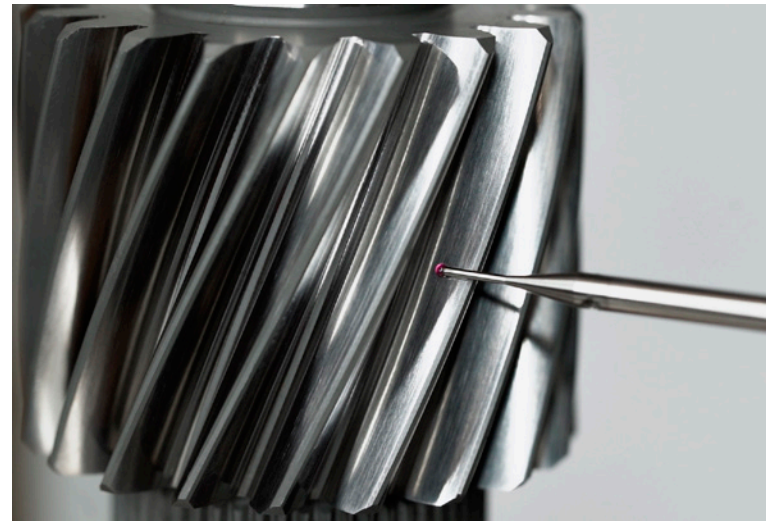
The 175GMS nano Gear Metrology System is equipped with a high-precision SP25 3D scanning probe head, a wide range of styli, and an advanced mathematical analysis that supports roughness evaluations to DIN, ISO, ANSI, and other standards.
