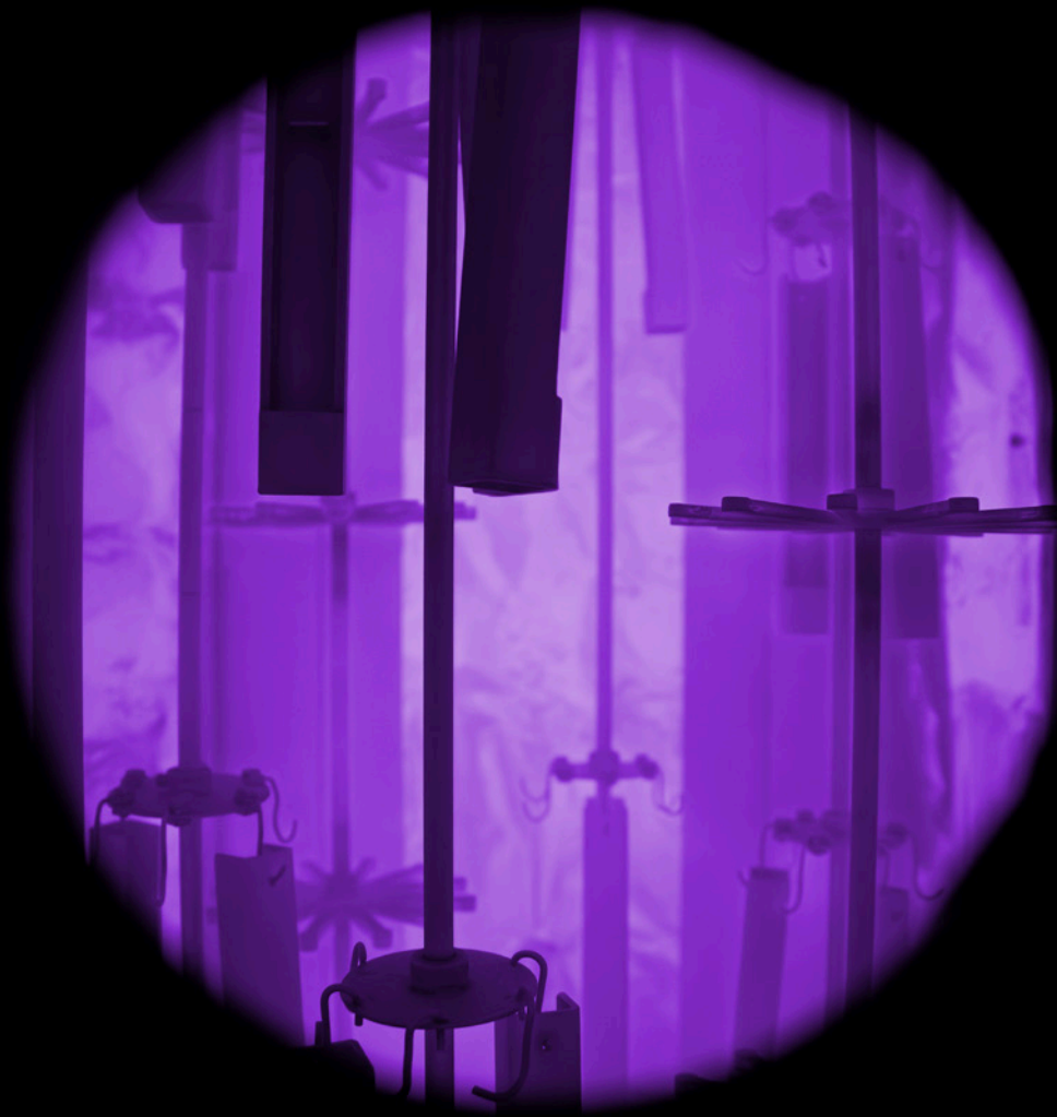
Figure 1—Parts being coated using PECVD.
