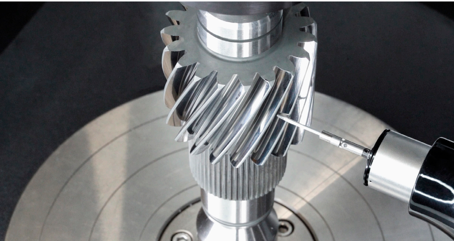
Users can now measure, at submicron level, gear pitch, tooth size, profile, and lead at high speed along with surface finishes with a skidless probe that is seamlessly integrated into the automated probe changer.
