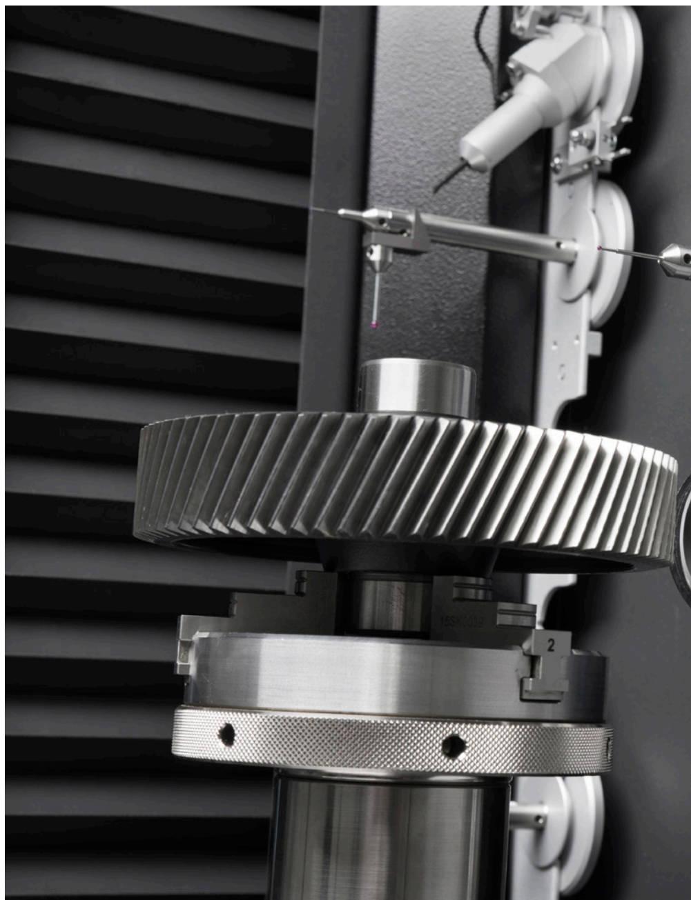
Figure 2—Hybrid metrology on a final drive for electromobility, gear quality 4 according to DIN ISO 1328, 82 teeth.
