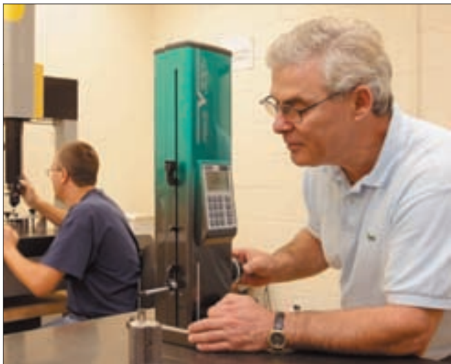
Precipart’s QC inspector Mihai Burucea (foreground) working at a digital height-gaging machine, while Ken Gentry monitors a CMM machine.
