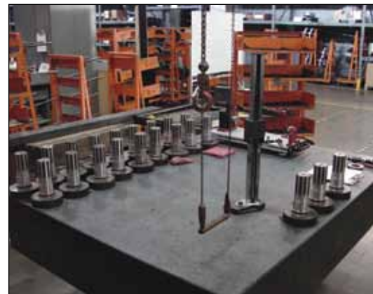
Cotta Transmission used the granite base of the old CMM as an inspection surface plate in its shop.
