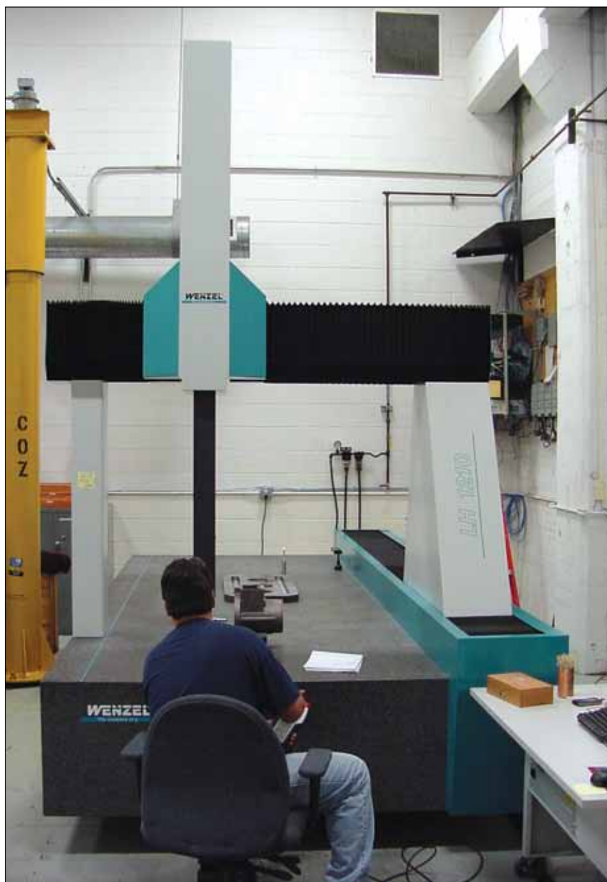
New Wenzel LH 12.30.10 bridge-type CMM installed at Cotta Transmission to inspect a wide range of industrial and commercial transmission components.
