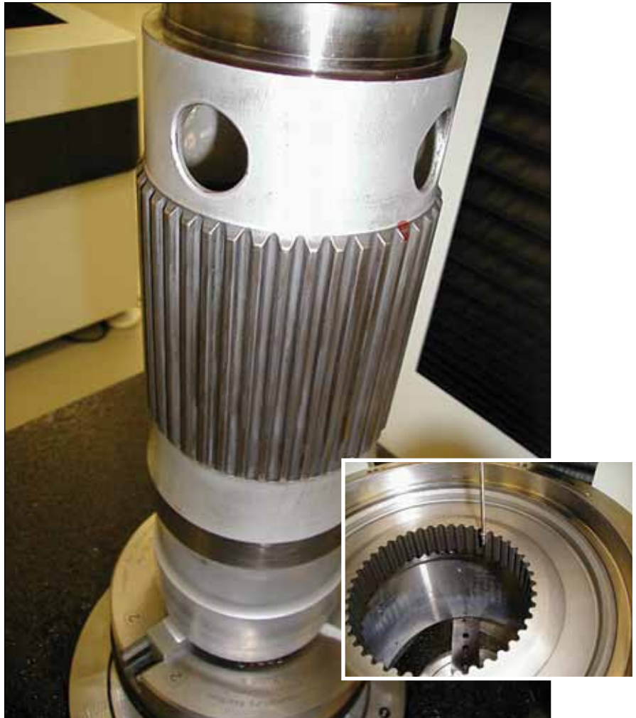
PECo's data acquisition and Renishaw 3-D probe technology enables the machine to generate measurements on various surfaces (All photos courtesy of PECo).
