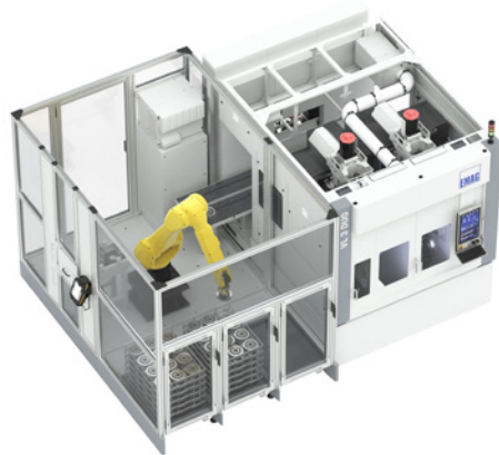
Figure 3—In automation cells with basket stacks, the system is loaded and unloaded by baskets from which the robot picks up or deposits the oriented workpieces. The empty baskets are transferred to the stack by the robot.
