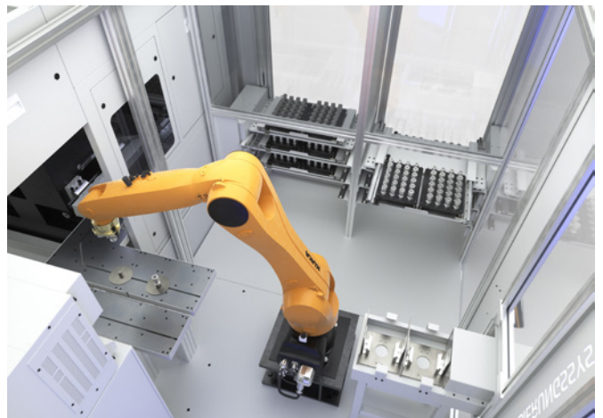
Figure 4—With the drawer system, the workpieces are provided to the robot on different levels. While the drawers are being loaded, the robot in the cell supplies the machine with workpieces.
