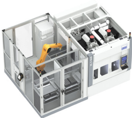
Figure 4—With the drawer system, the workpieces are provided to the robot on different levels. While the drawers are being loaded, the robot in the cell supplies the machine with workpieces.
