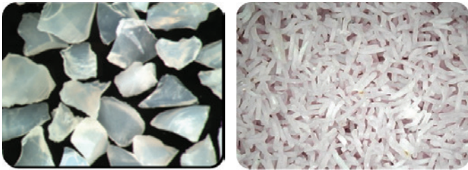
Figure 6—Norton angular and extruded ceramic grains.
