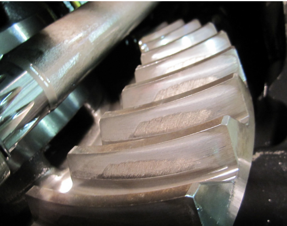
Figure 5—Scuffing in the root area of a hypoid pinion without profile shift.
