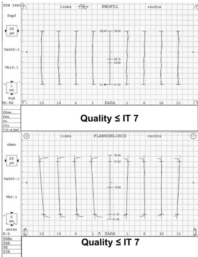
Figure 13—Final result hard-skived internal spline.
