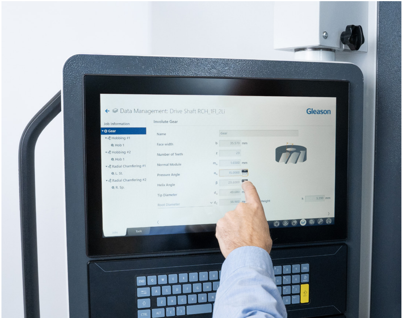
Coupled with the latest Siemens Sinumerik One control, Gleason's GEMS HMI hobbing software guides the operator intuitively through the workflows of the machine, both hobbing and radial chamfering.
