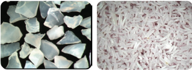
Figure 6—Norton angular and extruded ceramic grains.
