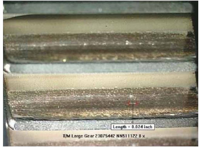
Figure 5—Baseline Gear B, Mesh 1: post-150-hour test.
