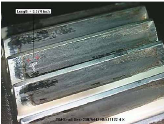
Figure 6—Baseline Gear C, Mesh 2: post-150-hour test.
