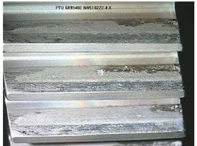
Figure 7—Baseline gear D, Mesh 2: post 150-hour test.
