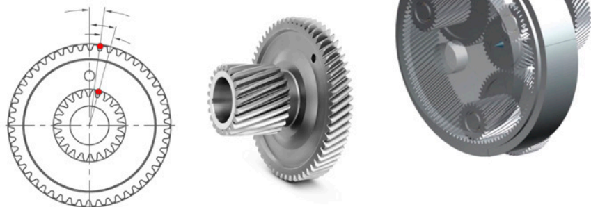
Figure 2—Synchronized stepped pinions with timing tolerance.
