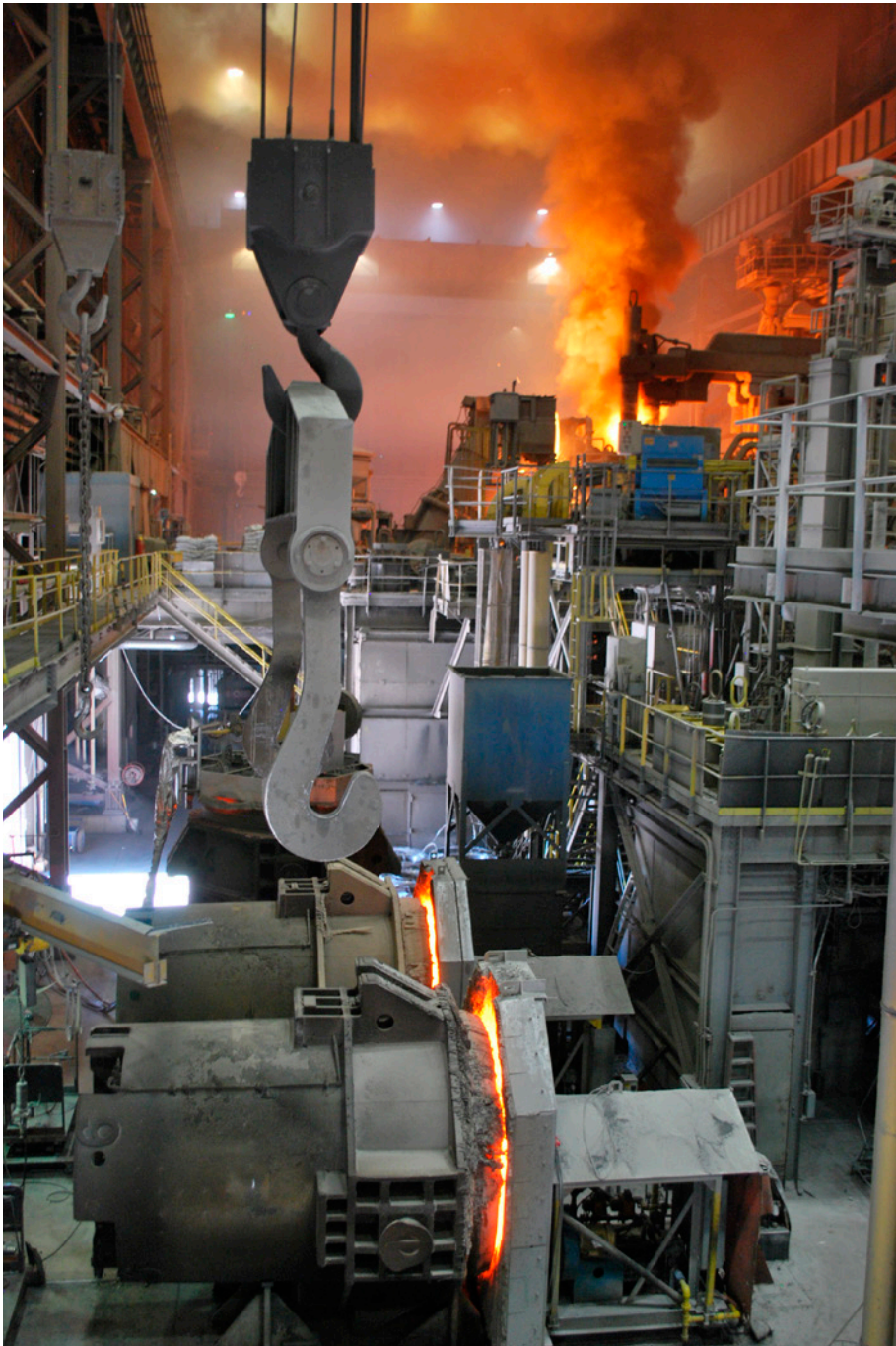
Argon rinsing at the ladle refining station promotes flotation of nonmetallic inclusions.
