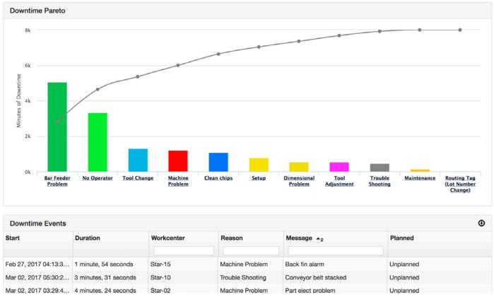
Figure 1-Pareto plot of capacity loss categories. Courtesy of MachineMetrics.
