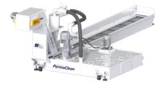
The EcoFilter 80 enables efficient filtration of fine chips to 80-microns nominal and is the first economical non-drum style conveyor below 100-micron filtration. EcoFilter conveyors use a two-stage chip removal and filtration process that carries out large chips on a hinged or scraper belt. Fine chips flow with used coolant between the belt runs to a flowthrough EcoFilter cell where they are separated from the coolant.
