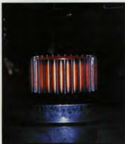
A near-net shape forged gear hot off the press. Courtesy of Presrite Corp.
