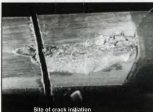
Fig. 7—Pitted gear tooth from the helical gear tests on Oil A. Note that the pit appears to have started from within the micropitted area.
