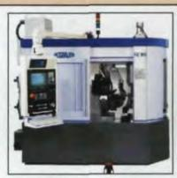
Technical data: Workpiece outside diameter 150 mm / 5.9" Number of teeth 6-150 Module/DP 1-3 / 25.4-8 Helix angle ±40° Workpiece weight maximum 3 kg / 6.6 lbs
