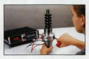
without a part, the addition of a "Power Control" unit assures extremely repeatable clamping of thin-wall parts without distortion. The system is extremely simple to use with the operator attaching 2 magnetic "paddles" to the arbor and actuating up to a pre-specified limit on the DRO. For more information, contact Euro-Tech Corporation at (262) 781-6777 or www.eurotechcorp.com.
