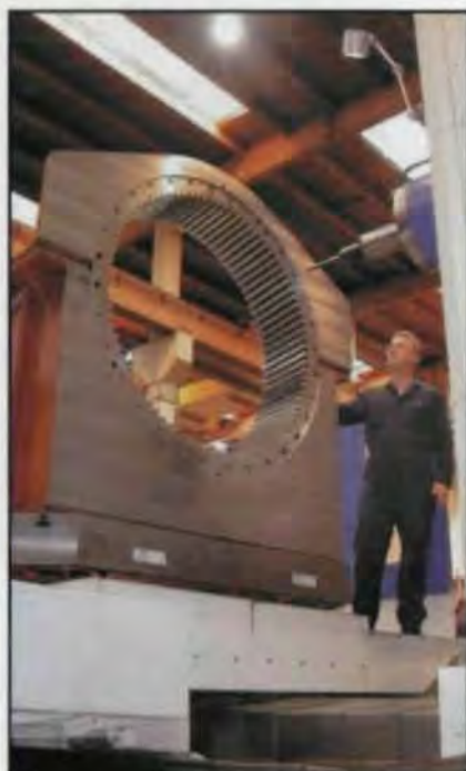
Internal ring gears for wind turbines generating 1.5-2.2 megawatts of electricity have 4- to 6-foot pitch diameters and AGMA quality levels of Q10-12.
