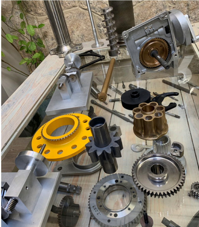
Forest City Gear's principal products are fine and medium-pitch custom gears, such as internal, spline, sprocket, helical, spur and worms/worm gears. Typical materials include 12L14, 1215, 4140, 8620, 9310 and various stainless grades, as well as aluminum, bronze, brass, Inconel, Hastelloy, titanium, plastics, wood fiber and powdered metal.
