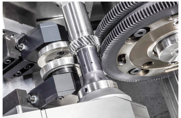
Chamfer rolling with secondary deburring discs. A very fast process that can, however, form a secondary burr that must be removed downstream.
