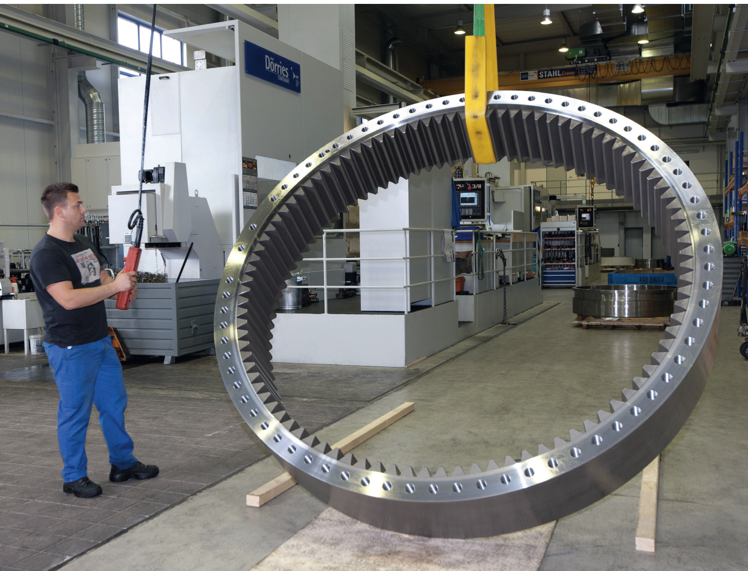
A large internal gear in production at Zahnradfertigung OTT GmbH & Co. KG.
